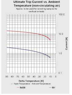
The curves of First Cycle Tripping time and Ultimate trip current are meant to be for selecting samples to perform verification tests only. In the figures two curves of a wide range of possibilities are shown. The level and slope can be varied by making an other selection for the pre-set temperature, bimetal disc and/or heater.
