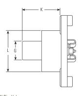
.065 ±.005/-.000 (.164 ±.254) Dia. Holes .062 ±.010 (1.57 ±.254) Deep (Type ME 4-Holes. Type CE 2-Holes at #1 Terminal End only. Other Types No Holes)
